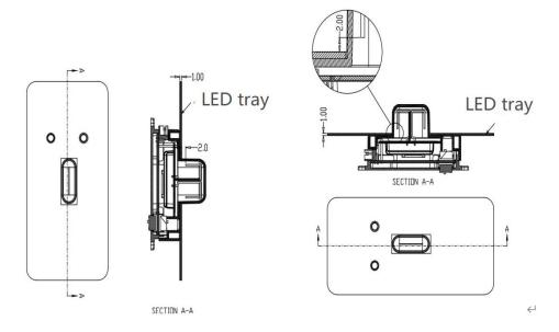
Note: Sensor antenna should be above LED tray at least 2mm.
