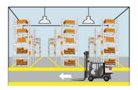
With sufficient ambient light, the light will not be switched on even if with motion signal.
