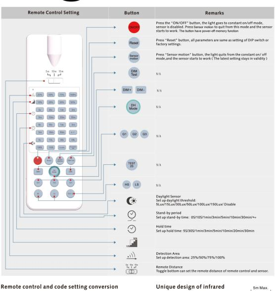
DIP switch setting convert to remote control Press any bottom except "RESET" on the remote control, and the sensor settings convert to the function currently selected by the remote control. (No function button settings invalid)
