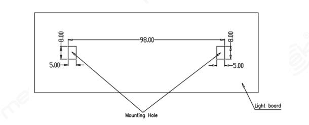
The mounting plate needs to be close to the top surface of the housing
