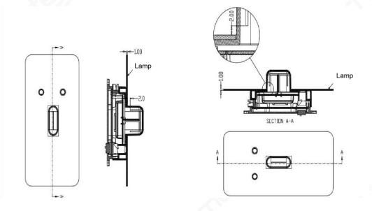
Suggestion: The bottom Angle of the light plate from the microwave antenna should be higher than 2mm, otherwise the induction distance will become closer
