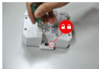
③ Use a screwdriver to pull the shrapnel into the lock position.
