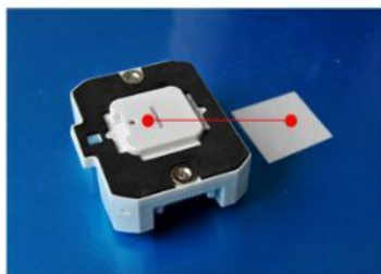
② Put the sensor in center of the hole ,and make sure the magnet attach to the cover firmly .
