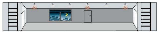
After stand-by period, the lamps will be switched off if no movement is detected in the detection zone.
