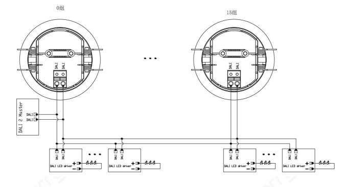
Remark: we recommend no more than 6pc sensor in a 250mA-circle to avoid communication problem due to insufficient loading problem
