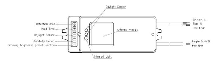
\*The sensor is designed for connect one load only. Connect more than one loads may damage the sensor.
