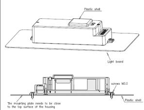
Cut the following buckle and using 2 screws.
