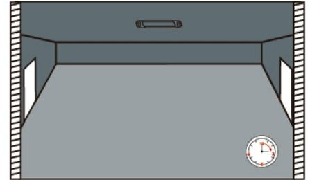
3 After elapse of hold time, the sensor switches off the light when no motion is detected.
