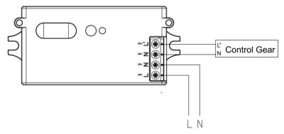
\*The sensor is designed for connect one load only. Connect more than one loads may damage the sensor.
