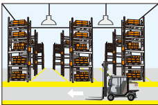
1. With sufficient ambient light, the light will not be switched on even if with motion signa.
